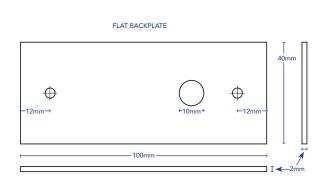
Parts - 1x Flat Backplate 2mm thickness, 2x 6Gx26mm Pan Head Screws
